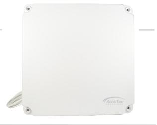
Radome Material: ABS Connector: RPSMA Plug Number of Leads: 4 Cable Length: 36" (910mm) Cable Type: ATS-195
